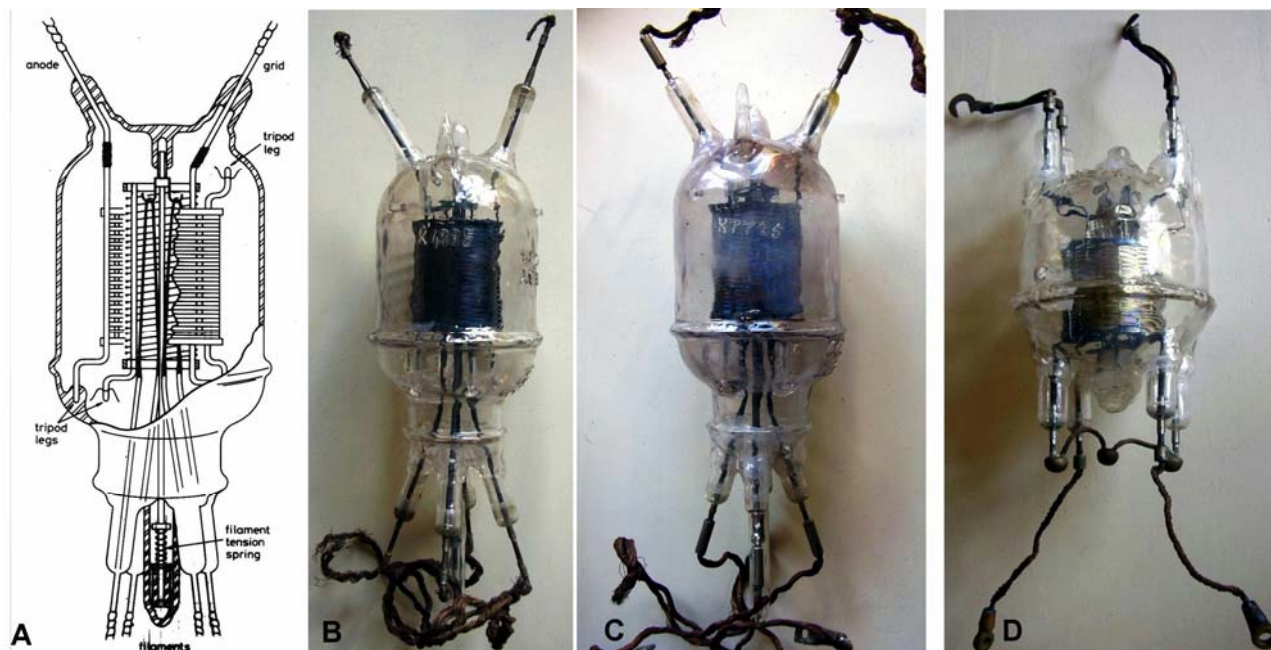
Fig. 8 - A) Drawing showing the construction of the NT57 triode, the first silica valve specifically designed for radar applications. Well spaced electrodes and divergent sealing legs grant low capacitance and high insulation. The thick double hairpin filamentary cathode gives 5 A minimum emission under pulsed conditions. B) The photo show a sample of NT57D , with short graded-glass seals, usable up to about 100 MHz. C) It was replaced from April 1939 by the NT57T with thoriated-tungsten filament, capable of delivering 18 A saturated emission, consuming less than half the power required by the filament of the previous one. In D) a sample of CV14 (XN), the latest of compact silica triodes proposed in 1941 to operate up to 240 MHz.
