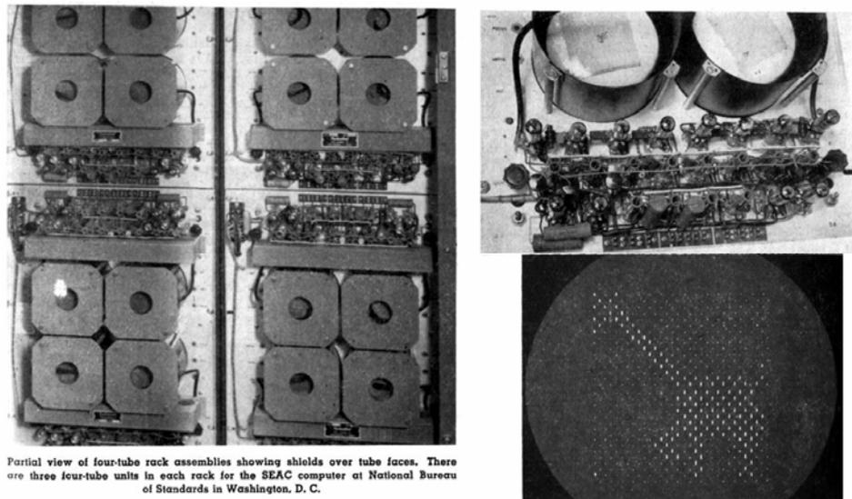
**Fig. 1 - Left, internal view of a CRT memory rack, showing groups of two CRTs, each with its associated Read/Write/Refresh circuitry. Right, a closeup view of two storage tubes with front shields removed and image of the memory content, as seen on the screen of an auxiliary monitor oscilloscope.**
