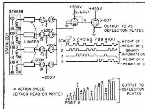
FIG. 8—Binary address digits are converted to weighted currents and summed before applied to plates
