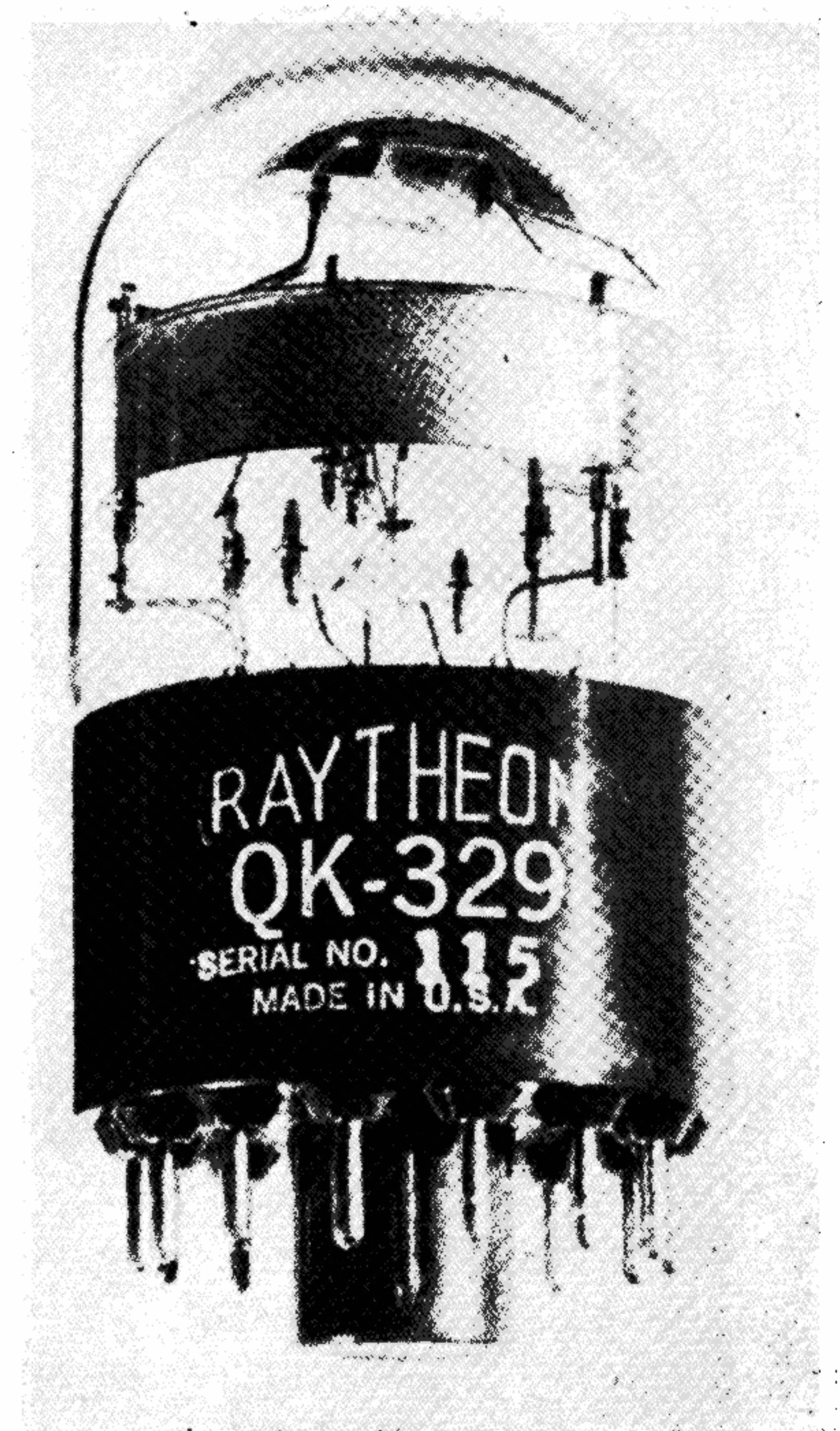
Type QK-329 beam-deflection tube provides full parabolic square-law action with 1 percent accuracy at full scale
