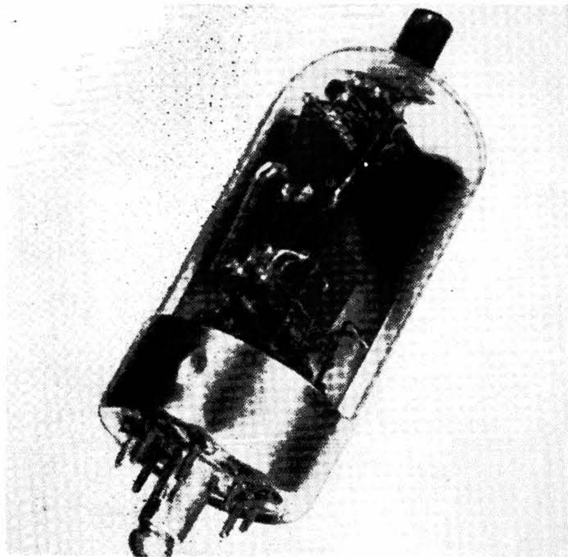
Anodyne tube utilizes T-9 bulb with grid cap
