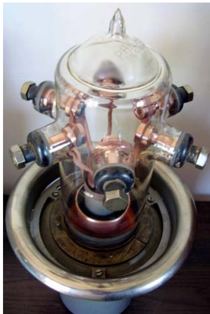
Fig. 4 - A very complex glass masterpiece with six radial spokes, sealed to heavy metal fed-throughs. The glass dome is then sealed to the copper anode below and evacuated from the top. Philips TAL-12/35 .
