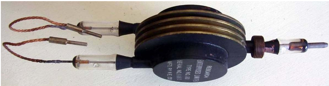
Fig. 18 - In this case the anode copper block is brazed to the internal wall of the brass finned radiator ring.
