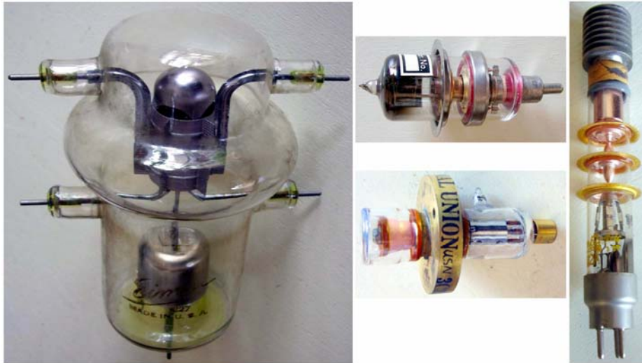
Fig. 5 - Other complex glass structures in high frequency tubes. Here high temperature glasses are precisely formed, assembled and sealed to very close tolerances, assuming a true structural function in supporting and spacing internal electrodes.
