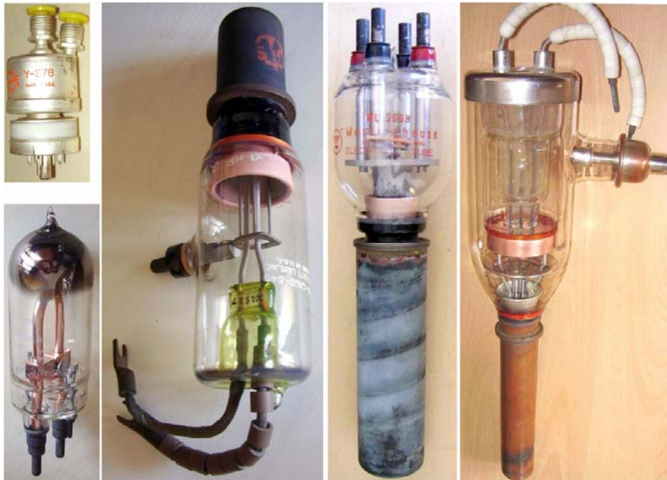
Fig. 19 - Water-cooled tubes. Top-left, a small VHF tube with integral heat exchanger. Bottom-left 5J29 , a split-anode magnetron fluid-cooled through the anode pins and the internal tuning loop. Other tubes are high power types in which copper anode is cooled by an external water jacket.
