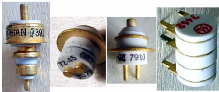
Fig. 6 - Due to the exceptional stability of ceramic materials used as spacers between electrodes, small triodes were made, capable of reliable operation up to about 10 GHz in extreme environmental conditions, up to 400°C, and even in strong radiation fields. 7077 , the second sample from left, was used in the Pioneer space probe. About 2x actual size. Here the GE Notes on these tubes.
