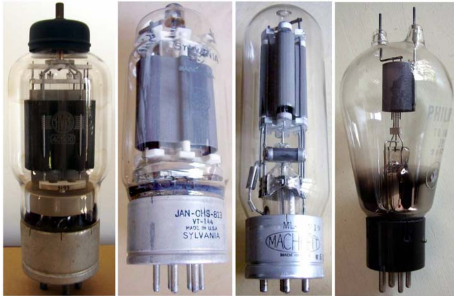
Fig. 15 - Graphite plates in transmitting tubes up to 500 W.
